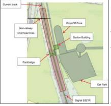
Phase 2 shows restoration of the double track between Fareham tunnel and Botley, with two platforms.
